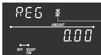
Electronic journal memory near end /memory full symbol
