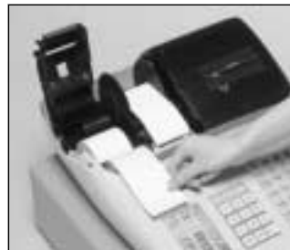
Step 4 Put the leading end of the paper over the printer.
