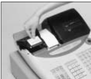
Step 2 Open the platen arm.
