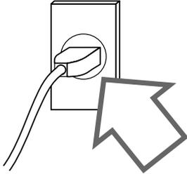
Be sure to check the sticker (rating plate) on the side of the cash register to make sure that its voltage matches that of the power supply in your area.
