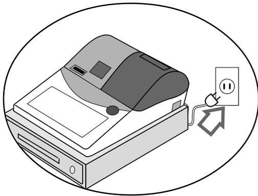
*Be sure to check the sticker on the side of the cash register to make sure that its voltage matches that of the power supply in the area.*
